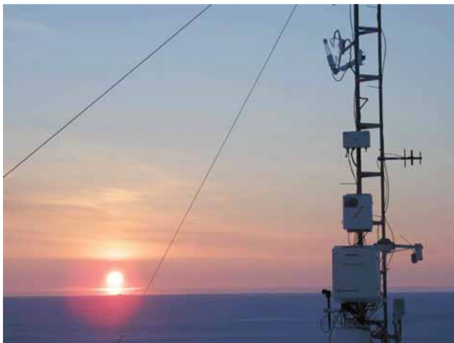
Figure 4. Eddy covariance system for measurements of CO 2 fluxes deployed over the sea ice (Franklin Bay, winter 2004). The sonic anemometer and open-path CO 2 detector are at the top of the picture. Credit: T. Papakyriakou
